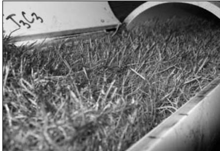
Maximum level of root occlusion in pilot system.
