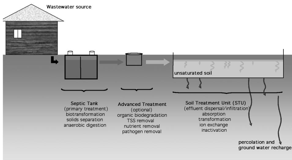
**Figure 1. Schematic of a Conventional OWTS with STU.**
