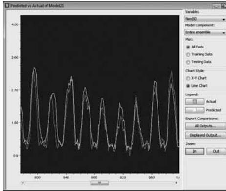
**Denitrification Model: Nine Days of Simulated and Measured Nitrate/Nitrite Concentrations.**
