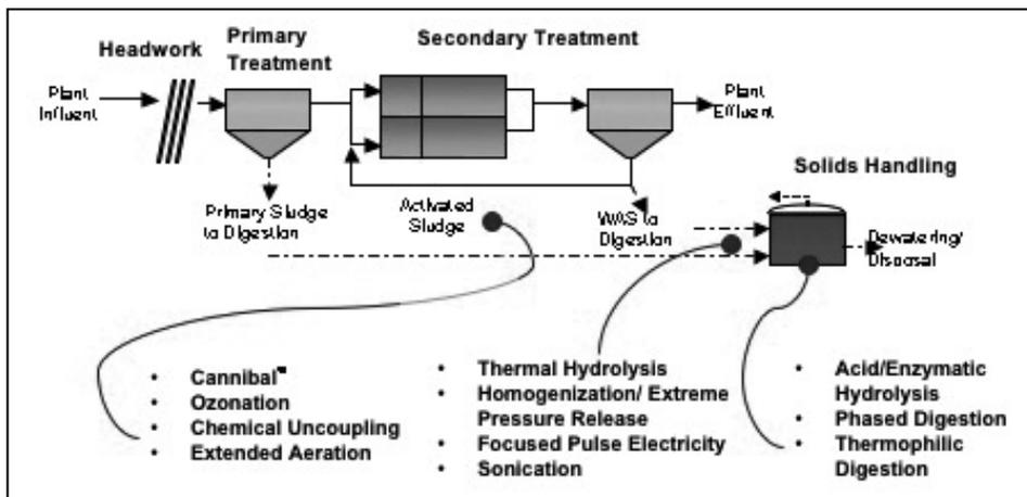
Figure 1. Examples of Waste Solids Reduction Technologies.
