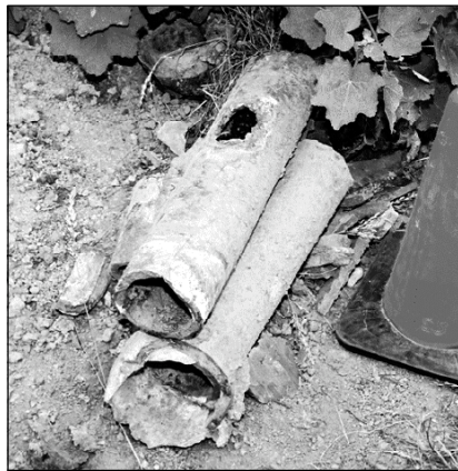
Example of the condition of laterals that were relined in Tacoma, Washington.
